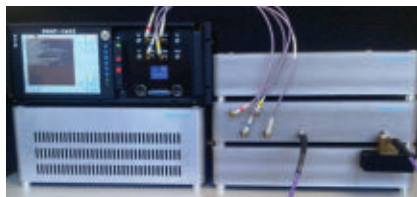
▲ Fig. 6 Setup for pulse time domain load-pull measurements.
