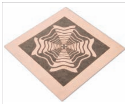
▲ Fig. 3 RF antenna structure made using the ProtoMat S103.
